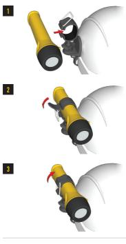
Position torch and lock by tightening nut.
