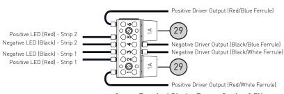
Output Terminal Block - Torque Setting 0.7Nm
