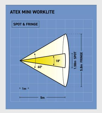
Spot Beam, approximately 18°, with a flood, approximately 60°, of lower level fringe light.
