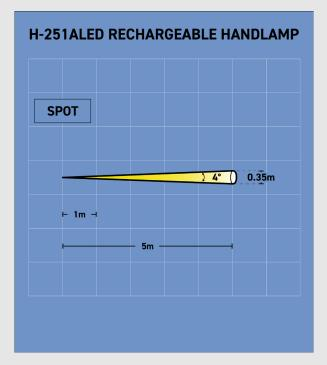
Spot Beam, approximately 4°, with a flood of lower level fringe light.
