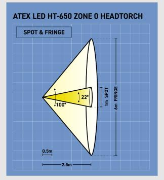
High Power LED spot beam (approx 22°) Peak luminous intensity at 1m 493 lux, at 2.5m 67 lux
