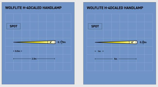
Spot Beam, Measuring at approximately 4° with a flood of lower level fringe light. 695 lux @ 5m
