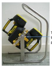
Tighten to lock in position
