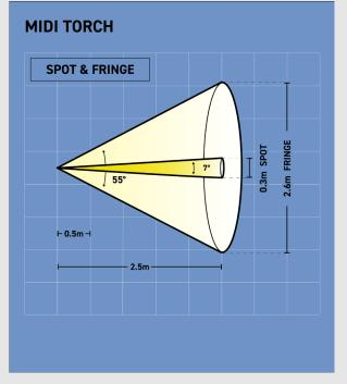
210 lumens LED **Spot Beam** (approx 7°) with a Wide Angle Fringe Beam (approx 55°) Peak luminous intensity at 1m **6500 lux**, at 2.5 m **1233 lux**
